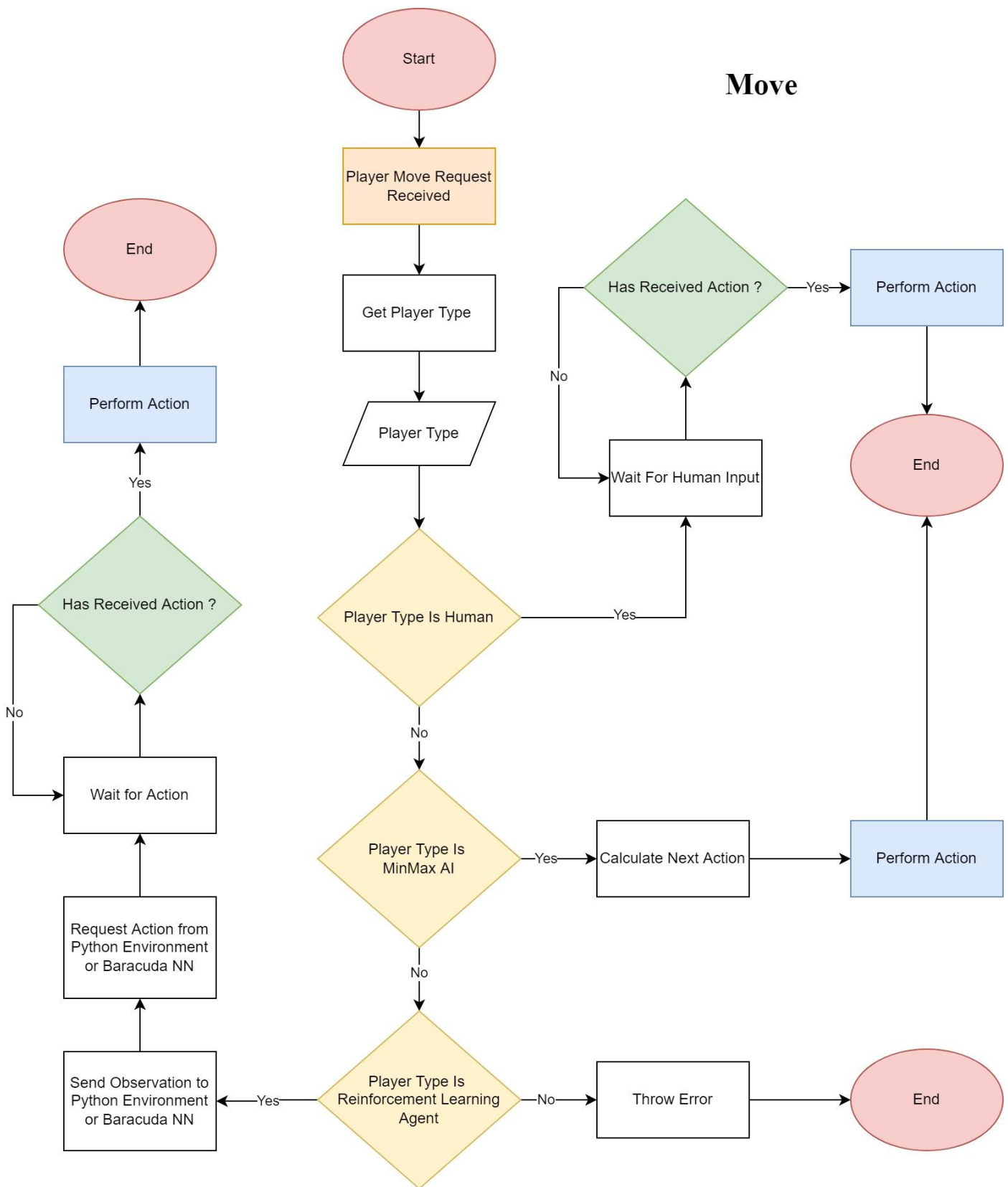
Figure 3.2 Basic Process of an Action
